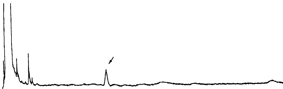
Figure 2 Chromatogram of heptaoxyethylene dodecylether (HOE) in Kengun river water
